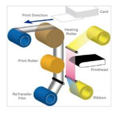
ReTransfer print technology is the next level up to Direct-To-Card print technology. First, the image is printed on a film, then transferred from the film to the card. This technique is suitable for Over the Edge, Heavy Duty Printing, improves reliability and is suitable for a vast variety of card types, such as:
