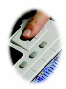
The 500dpi fingerprint sensor allows you to capture a high quality image to positively match identity.
