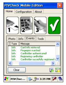
Once the card is removed, the *Photo* and *Info* tabs are cleared. The card reader icon appears in color, signaling the system is prepared to validate a new card.
