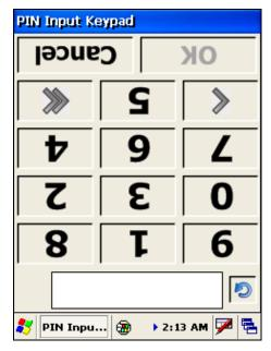
The PIN pad can be transposed to support the point of view of the operator by pressing the circular blue arrow.
