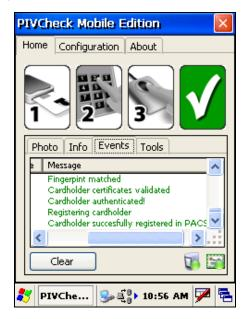
Once the card is re moved, the *Photo* and *Info* tabs are cleared. The card re adericon re-appears in color, signaling the system is prepared to validate a new card.
