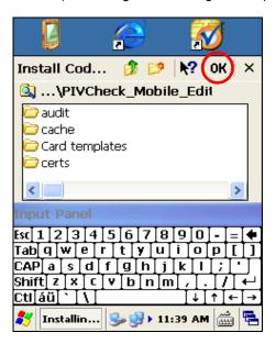
Tap the *OK* button to proceed with the installation. The progress bar will appear to be truncated at both ends. This is normal Windows CE behavior.
