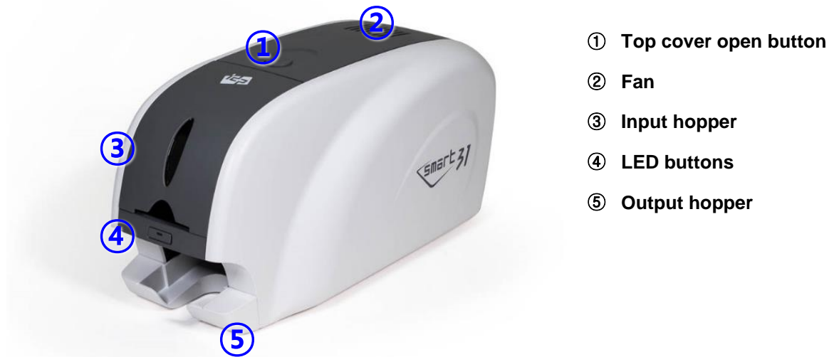
Figure 1 SMART-31 front features
