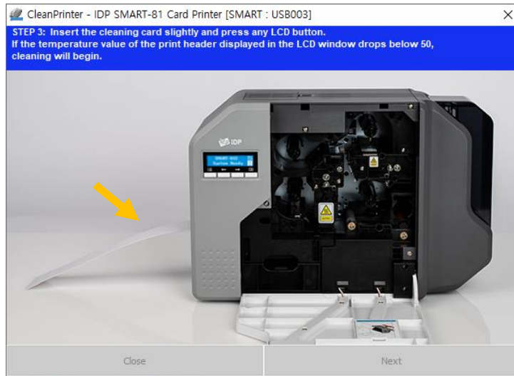
Figure 90 Printer cleaning step 3
