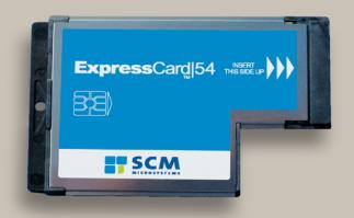
The SCR3340 is available for built-in integration into notebooks, PDAs, Thin-Client systems, and ExpressCard/54™ Adapters for PC systems.
