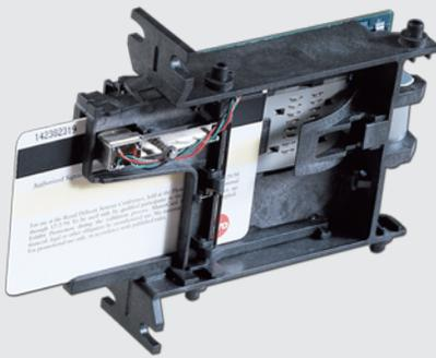
The FS65 not only excels in applications for unattended transactions, it also integrates a magnetic card reader with a smart card reader in a modular and compact design.
