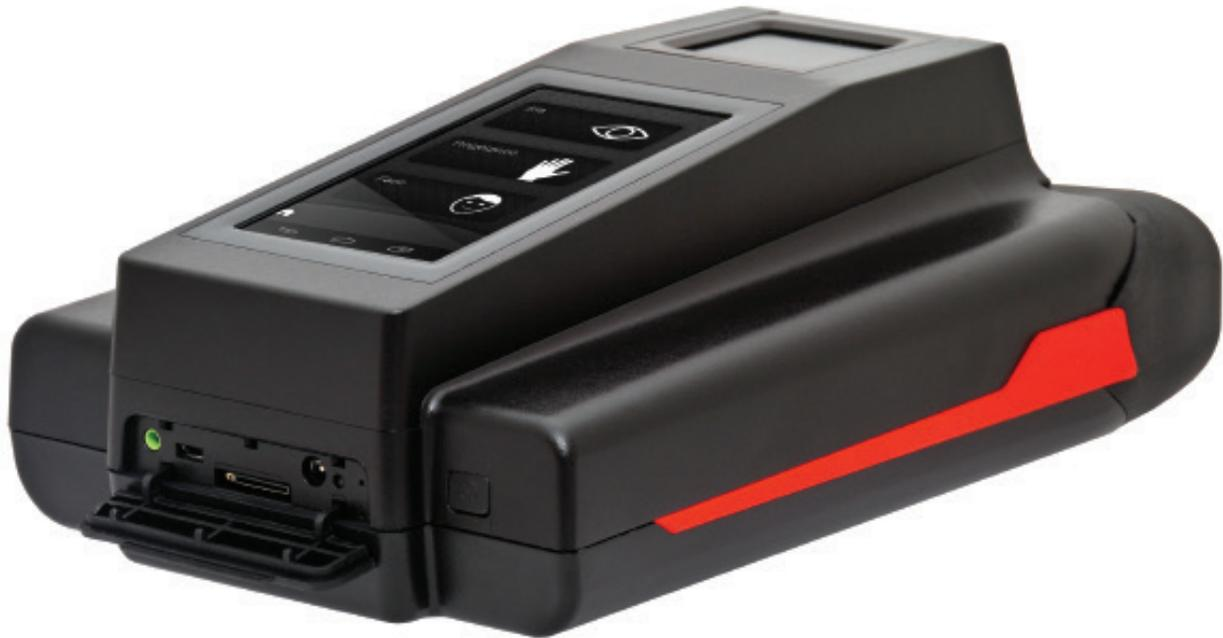
Trident is a completely integrated multi modal mobile biometrics device that combines the world's smallest and fastest FAP 45 fingerprint scanner, the world's first binocular-type iris capture on a mobile device and a stunning five MP auto-focus camera with flash. Trident runs on the latest Android 6.0 OS, widely deployed and proven mobile operating system.
