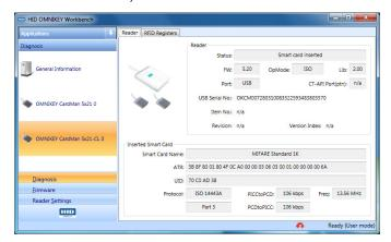
For a functional test, insert a working smart card into the reader. As a result, an ATR string and other card details will display.
